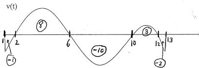
A particle moves horizontally so that its velocity at time t, for  $1 \le t \le 13$  is given by a differentiable function v whose graph is shown above. The velocity is 0 at t = 2, 6, 10 and 12 and the graph has horizontal tangents at t = 4, 8, and 11.
