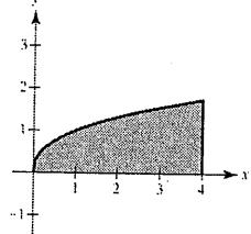
$$(a) \text{ Around } x\text{-axis: } V = \pi \int_0^4 (x^{2/5})^2 dx = \left[ \pi \frac{5}{9} x^{9/5} \right]_0^4 = \frac{5}{9} \pi (4)^{9/5} \approx 6.7365\pi$$
