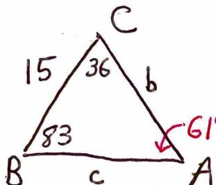
$$\begin{aligned} \frac{b}{\sin 83^\circ} &= \frac{15}{\sin 61^\circ} & \frac{c}{\sin 36^\circ} &= \frac{15}{\sin 61^\circ} \\ b &= \frac{15 \sin 83^\circ}{\sin 61^\circ} & c &= \frac{15 \sin 36^\circ}{\sin 61^\circ} \\ b &= 17.022 & c &= 10.081 \end{aligned}$$
